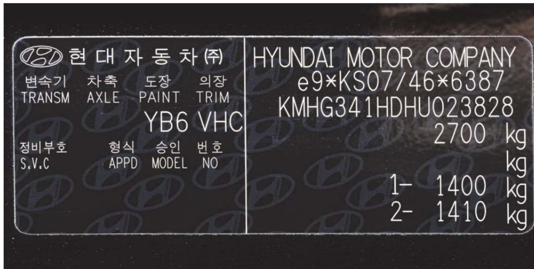
Fig. 3 Demonstration of an optical variable element – Hyundai logo, which is visible only under a certain light angle. In the logo (right leg of the letter H), an additional “micro-text” element is also used, which contains the word “Hyundai”.
