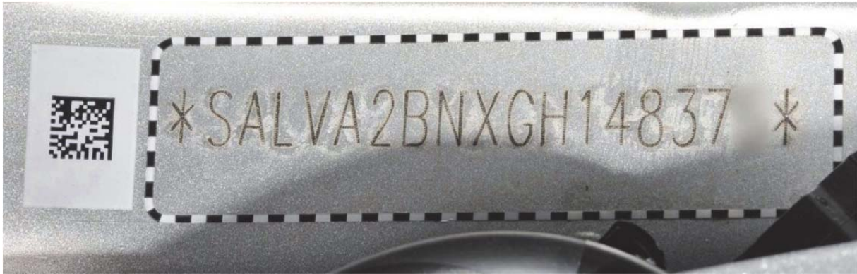
Fig. 5 Demonstration of the protective transparent cover foil of a stamped VIN identifier of a Range Rover vehicle.
