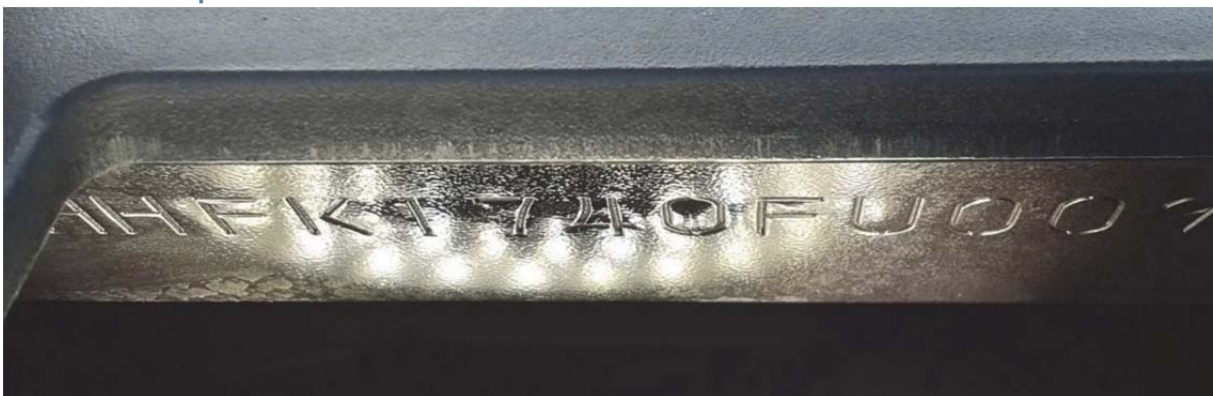
Figure 4. Overall, the identifier is visually inaccessible even following this dismantlement. Reading the VIN is very uncomfortable, and the inclined surface plays a role as well.
