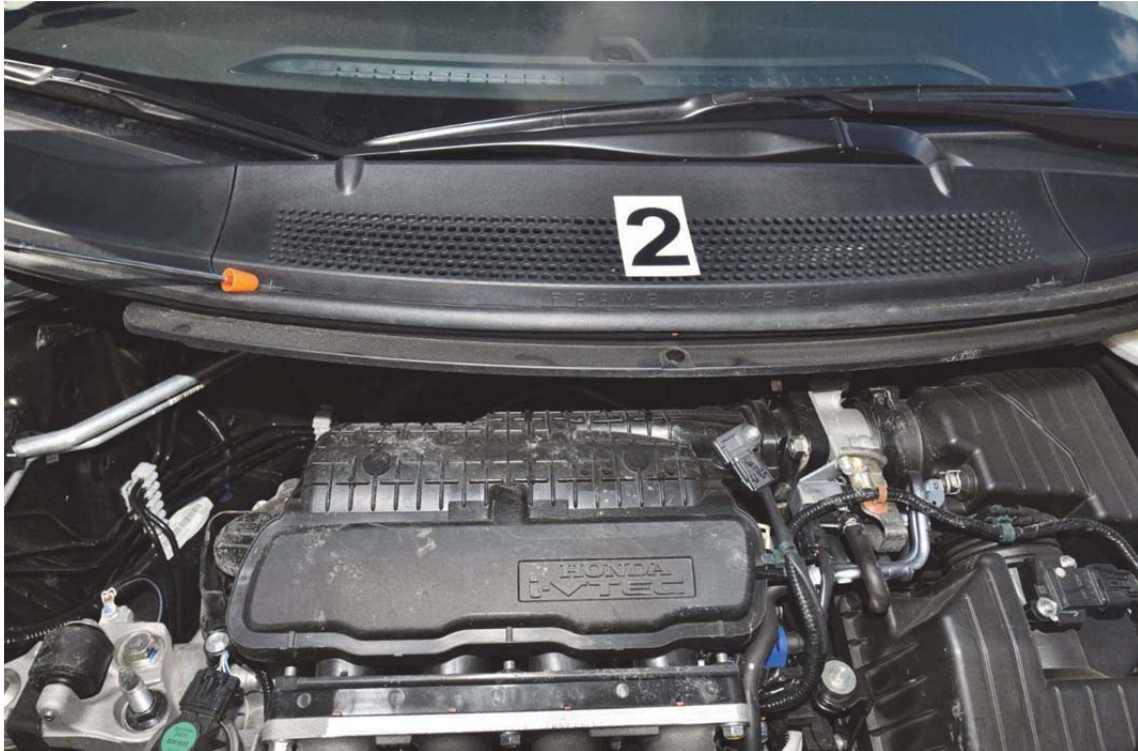
Figure 2. Example of a difficult-to-access VIN in a Honda Civic vehicle. For the identifier to be visually accessible, plastic parts must be expertly dismantled.
