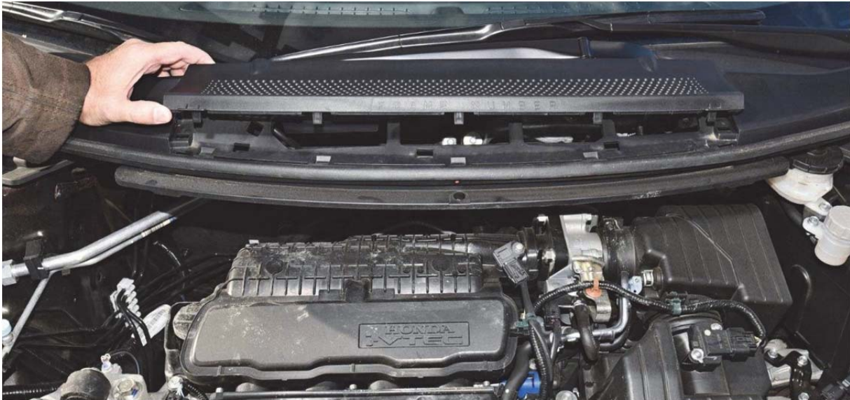
Figure 3. Demonstration of a dismantled plastic cover in the space in front of the windscreen wipers.
