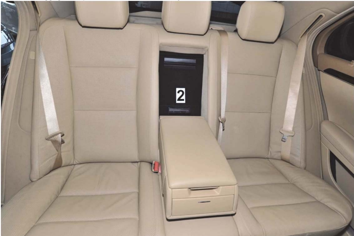
Figure 6. A VIN located in a non-standard way in a Mercedes – Benz “S” class vehicle in the space behind the elbow rest of the rear seats. It occurs to hardly anyone to look for the identifier there. On the other hand, this space is clean, dust-free so the identifier is not exposed to the negative effects of ambient phenomena.
