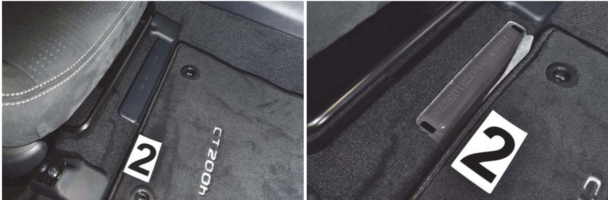
Figure 7. The VIN of a Lexus CT 200h vehicle standardly placed below the front passenger's seat. The VIN is protected by a plastic guard against damage and soiling.
