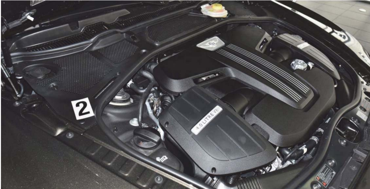
Figure 1. A standard VIN position in the engine compartment of a Bentley Continental GT vehicle. The VIN is easily visually accessible (to the right from the number "2").
