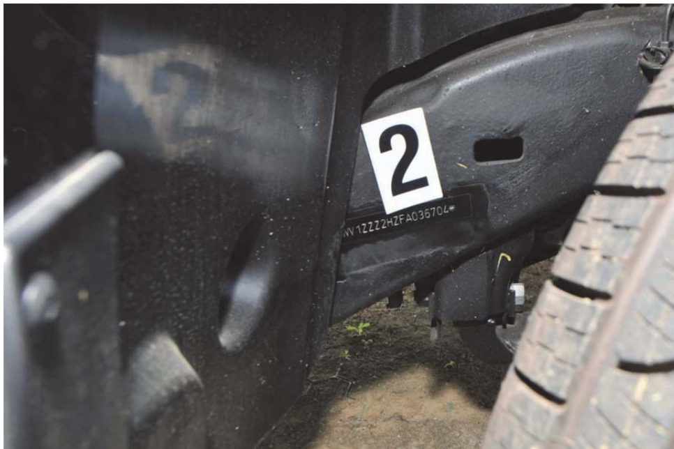
Figure 9. Volkswagen Amarok. The VIN identifier is located outside the vehicle on its chassis part and is protected by a transparent cover label. Placing the VIN in this part of the vehicle is not too fortunate – comfortable for practical inspection (one has to bend down and, at the same time, turn the wheels), the vehicle chassis tends to be very heavily fouled, so one has to know exactly where to look for the identifier. After several years of operation, the identifier is severely corroded, so its legibility decreases abruptly.
